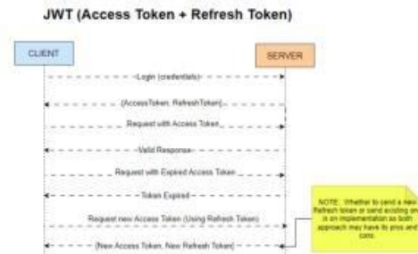
Figure 3.2: JWT Authentication Workflow in Node.js and C#
